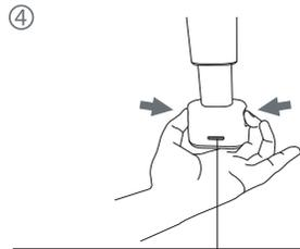
빨간색 In red → 초록색(바른 장착 표시) In Green (Indicated mark in correct)
